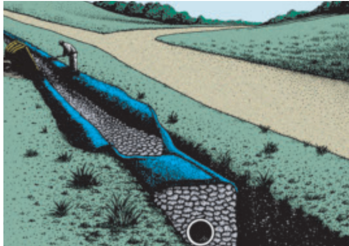
Wrapping a subsurface drainage system with a Propex nonwoven geotextile will improve roadway life.
